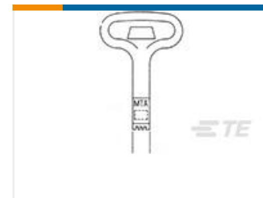
TE Part # 59804-1 MAINTENANCE TOOL
